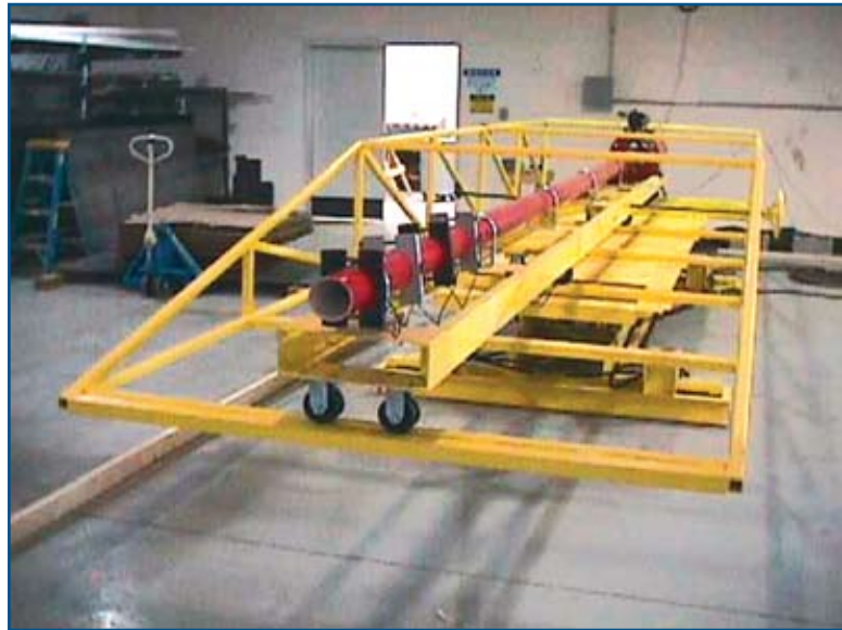
Missile (debris) launcher, Wind Engineering Research Center (WERC), Texas Tech University
